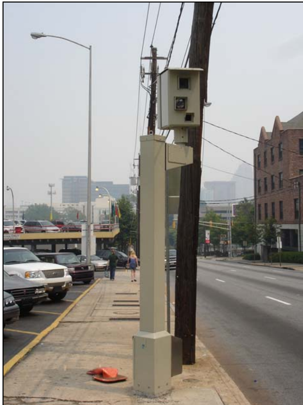
Figure 10. Gatso RLR camera system (Atlanta, GA).
