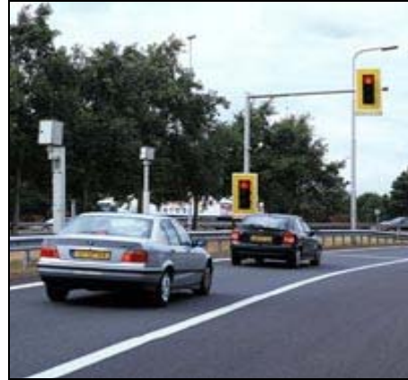
Figure 9. Gatsco RLR camera system (31).
