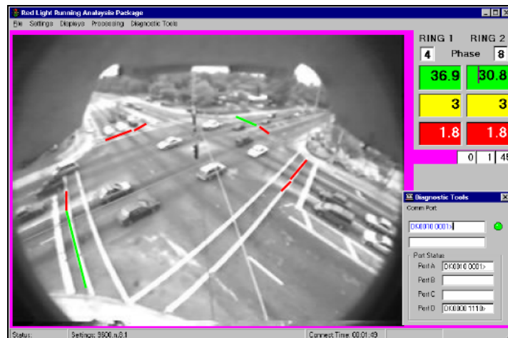
Figure 18. RLRAP monitoring an intersection (58).
